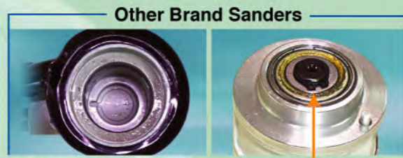
Mechanism tested for 1 hour Grease leaks seriously
